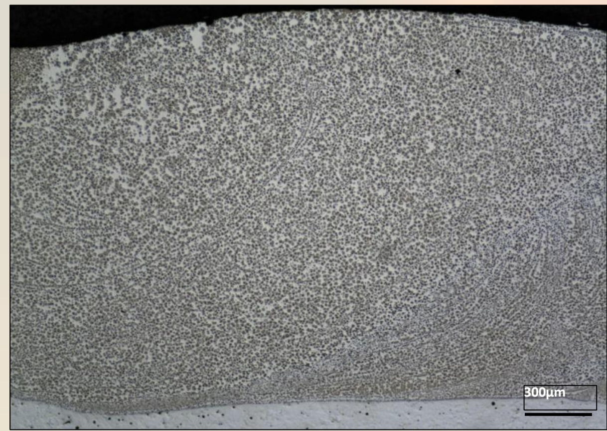
Typical Lasercarb® overlay cross-section of R706
